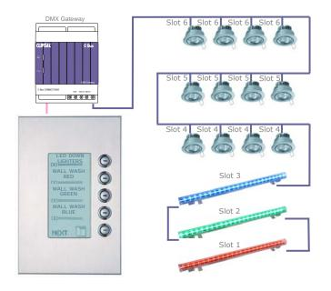
In a DMX-512-A network, multiple devices can be configured onto the same Slot Address. Therefore loads that follow the same control pattern can be controlled from a single C-Bus Group Address.
