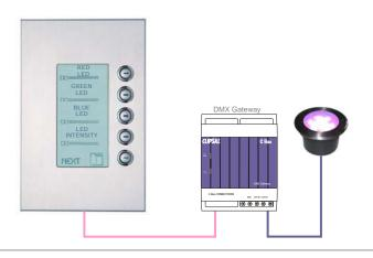
Some DMX-512-A devices may use multiple DMX-512-A Slots for colour and intensity control. For instance some LED devices use one DMX Slot Address each for Red, Green, Blue and intensity.
