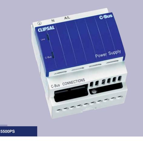
The C-Bus® Power Supply Unit supplies C-Bus power to passive C-Bus® units such as Key Inputs and Occupancy Sensors. For ease of installation the units are DIN rail mounted measuring 4 DIN modules wide.
